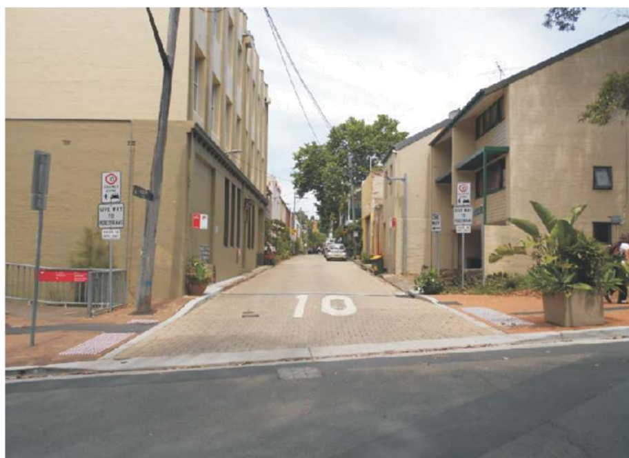
Figure 1. Photo and diagram of a Category 1 shared zone showing regulatory signage, typical layout and treatments. [Note: The No Entry sign is site specific] The photo may have been modified to demonstrate essential elements.
