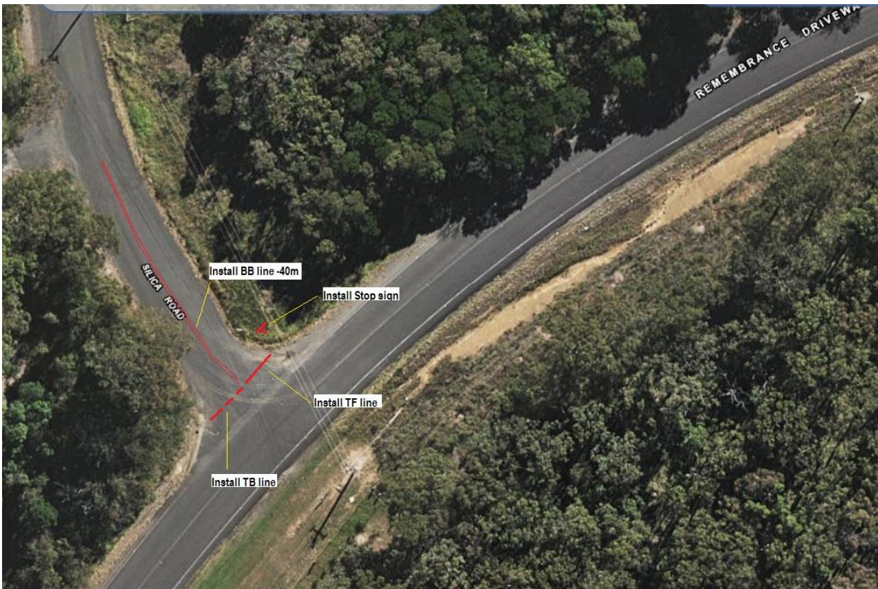
Proposed installation of Stop sign and linemarking at Silica Road and Remembrance Driveway T-Junction.
