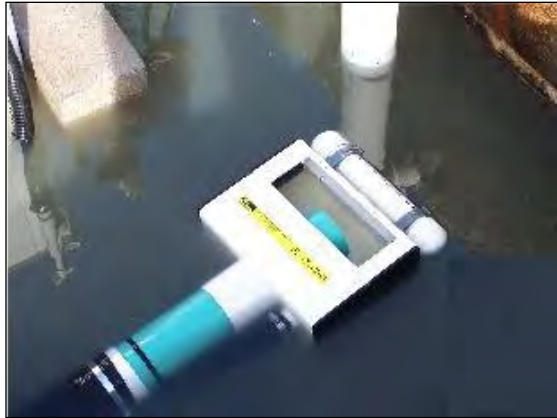
Figure 14.6 The Flout® is free floating
