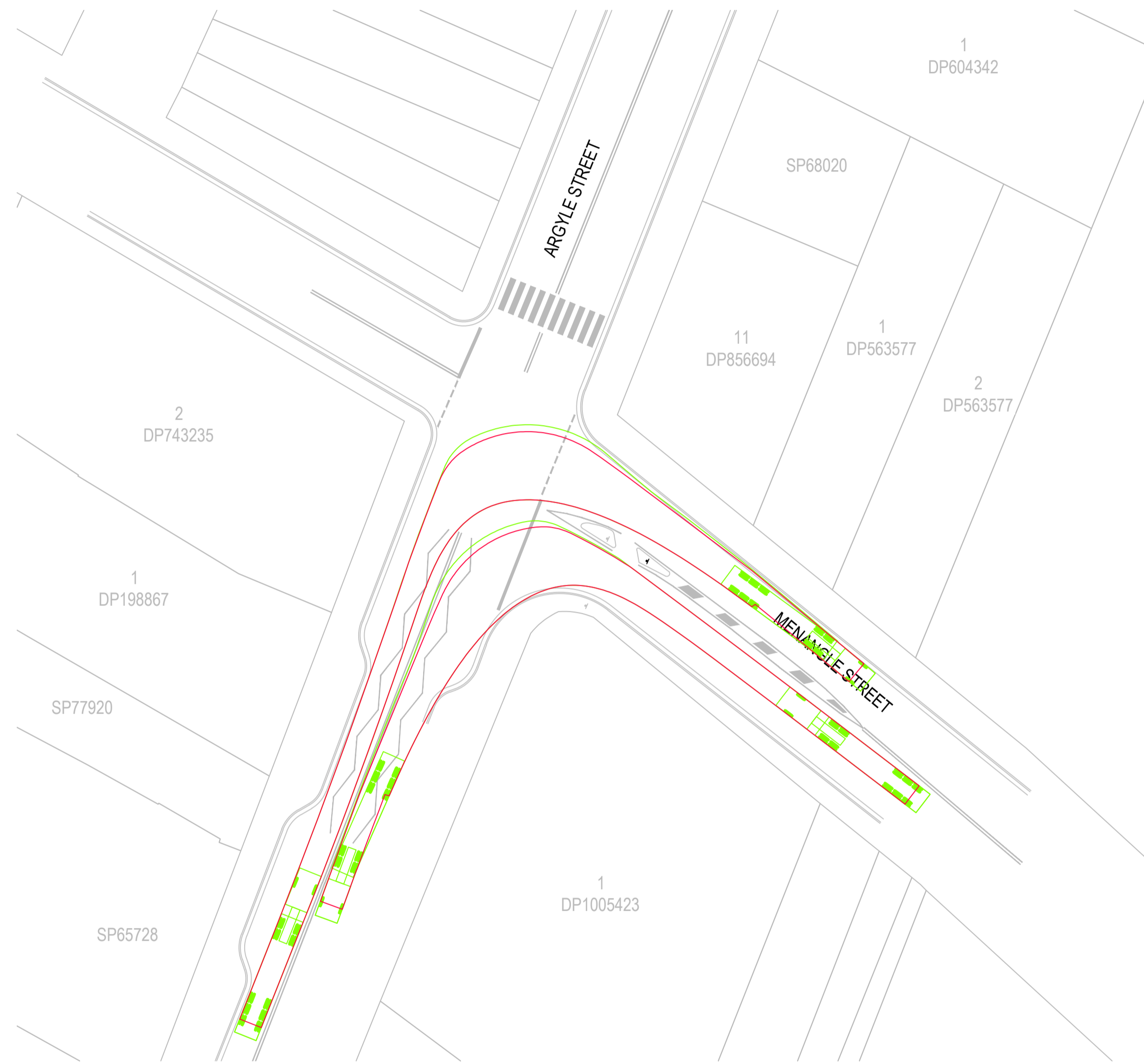
PRELIMINARY ARGYLE AND MENANGLE STREET INTERSECTION VEHICLE PATHS SCALE 1:400
