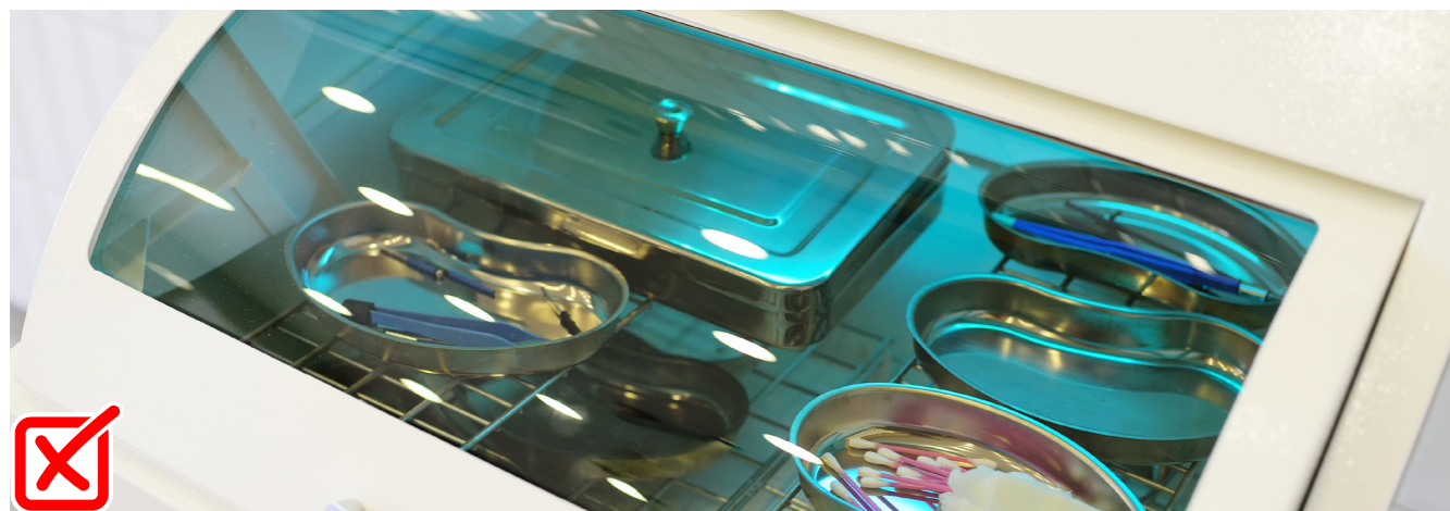
UV light cabinet is NOT an autoclave and does not sterilise equipment
