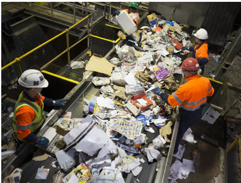
Figure 7: Material separation at a domestic recyclables resource recovery centre
