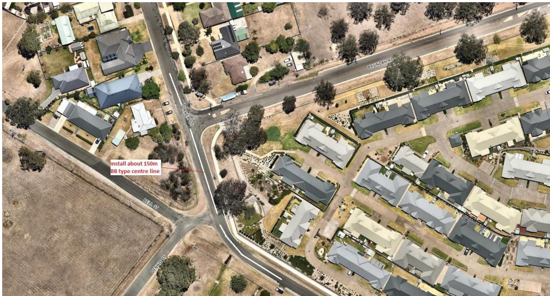
Proposed BB Type centre line marking on section of Turner Street – Bell Street
