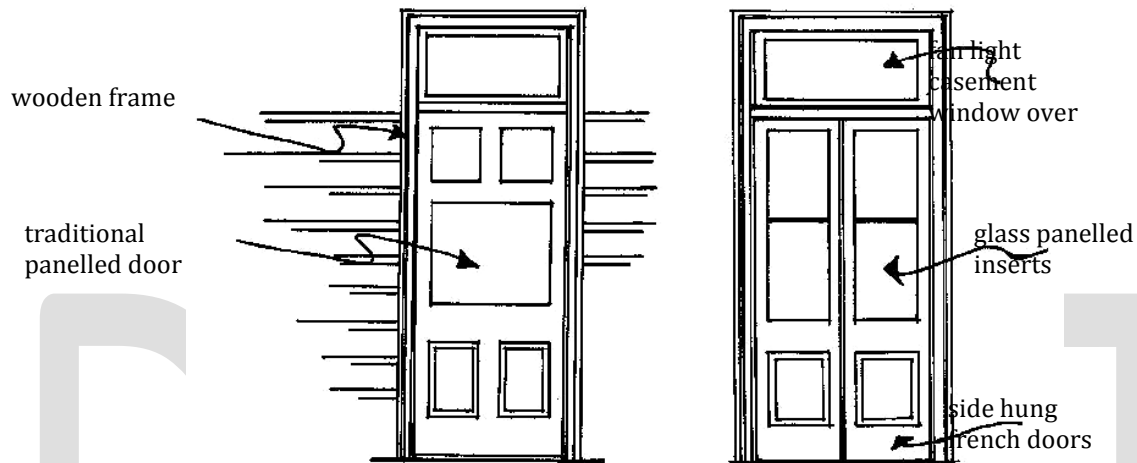
Figure 3 – Doors used in Early 20th Century Dwellings
