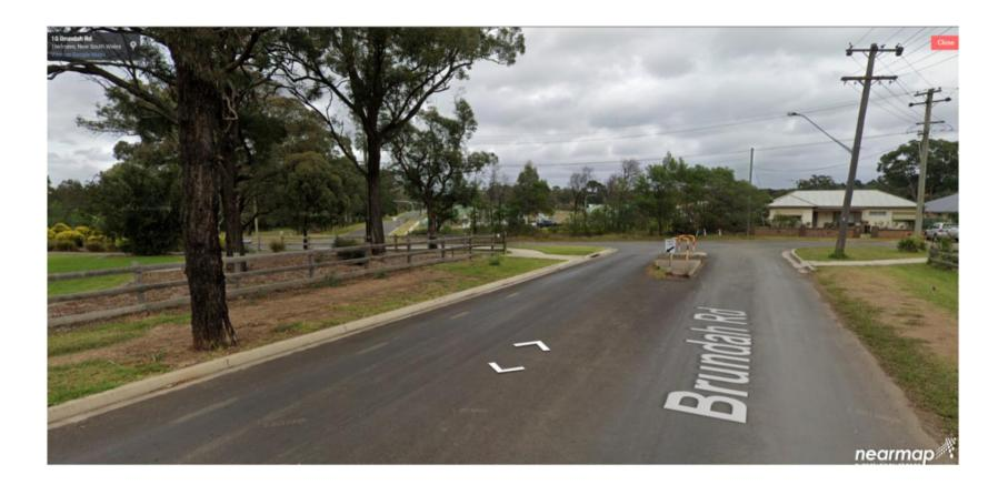
1.3 DOUGLAS PARK DRIVE, DOUGLAS PARK - PROPOSED 370M OF YELLOW UNBROKEN (CONTINUOUS) EDGE LINES ON SECTION OF THE ROAD BETWEEN 40M NORTH OF THE CAUSEWAY TO 280M SOUTH OF THE CAUSEWAY OVER NEPEAN RIVER
